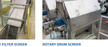
As the drum rotates, screened fluids pass through the perforations in the drum and fall into the water collection trough underneath the drum and are then discharged. Solids are retained within the drum and are dewatered as they are moved to the elevated end of the drum by the internal flights.
