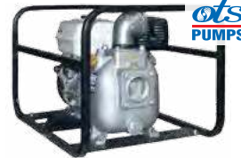
O Series® Engine driven utility Size: 3" (75 mm) Power: Honda - Gasoline Max Capacity: 400 GPM (25.2 lps) Max Head: 160' (48.8 m) Materials of Construction: Copper Alloy, Aluminum or Steel Impeller, Ductile Iron or Cast Steel Housing
