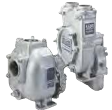
O Series® Power take-off or hydraulic motor driven Size: 2" (50 mm) to 3" (75 mm) Max Capacity: 400 GPM (25.2 lps) Max Head: 440' (134.1 m) Seal Elastomer: Viton® Materials of Construction: Copper Alloy, Aluminum or Steel Impeller, Ductile Iron or Cast Steel Housing
